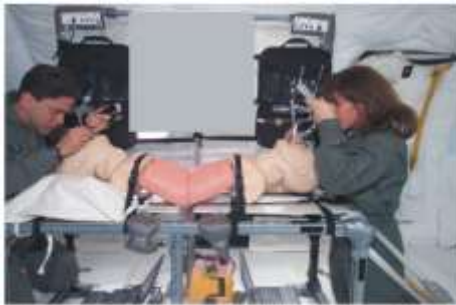
Fig. 1. Experimental apparatus showing the frame holding the two mannequins and the two flyers.
