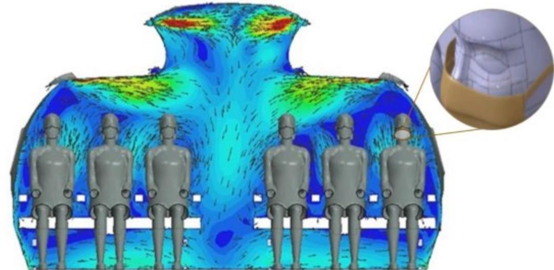
High quality full 3D Computational Fluid Dynamic models of cabin air flow, correlated with aircraft test-data and physical ground tests
